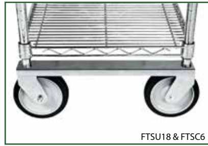
Caster channels are made from 304 stainless steel. 6" Polyurethane stem casters feature heavy duty stainless axles. Weight capacity per caster is 400 lbs (182 kg).
